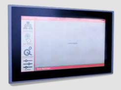
The HAFSTalpha is the latest generation of semiautomatic color controllers from OLIGO Lichttechnik GmbH – surface controls. Light scenarios and light groups can be quickly and conveniently configured via a TFT touchscreen display. A large overview display of the color matching booth visualizes the settings that have been made.
